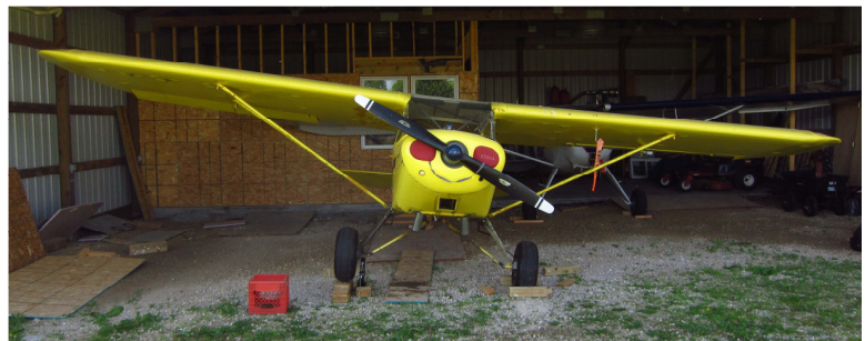
Figure 10: Calibrating unit by jacking the aircraft to each ball position
